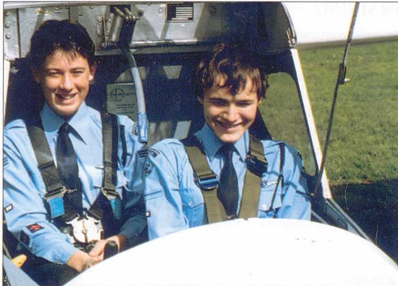
A Schneider “Kookaburra”, with staggered side-by-side seating, the right-hand seat being about 35 cm behind the left-hand seat
