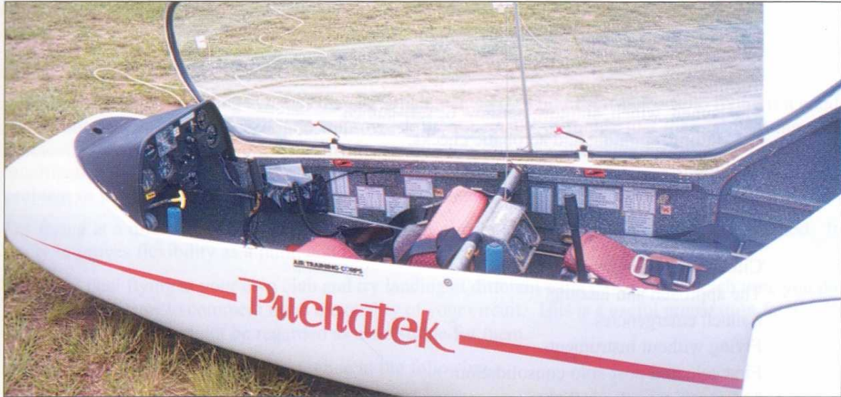
The cockpits of the Polish KR-03A “Puchatek” tandem two-seat trainer
