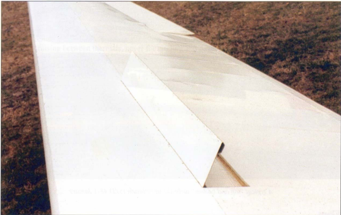
A typical spoiler installation (Scheibe SF25 "Falke" powered sailplane)
