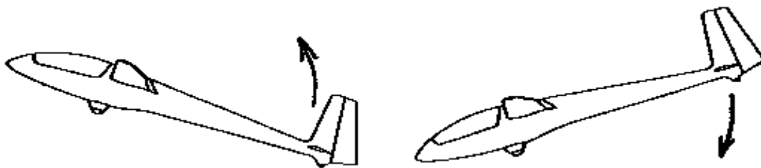
The tailplane provides pitch stability
